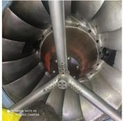
Belzona 1111 used to repair and Belzona 1341N used to protect the perimeter area of the cone.
