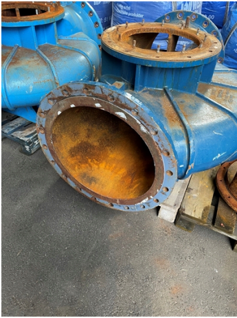
Corroded pump housings
