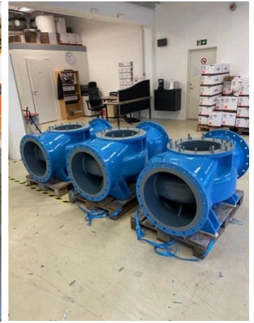
Coating application completed.
