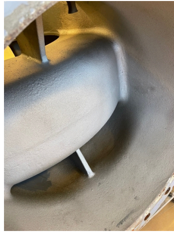
Grit blasted details
