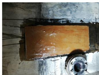
Ebonite tank suffering from degradation
