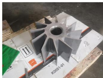
The impeller rebuilt with Belzona 4301
