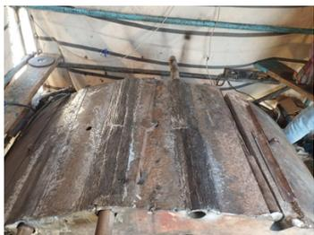
Damaged ball mill surface
