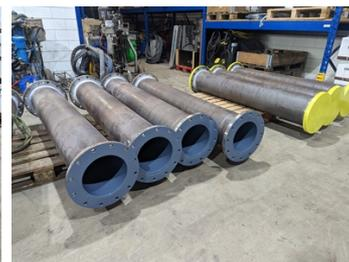
Second coat of Belzona 5821 in slate grey applied
