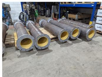
First coat of Belzona 5821 in yellow applied to pipe straights
