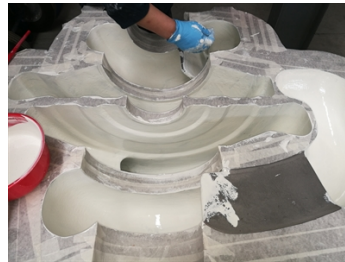
During application of Belzona 5811 DW2
