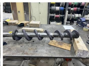
After application of Belzona 1812.
