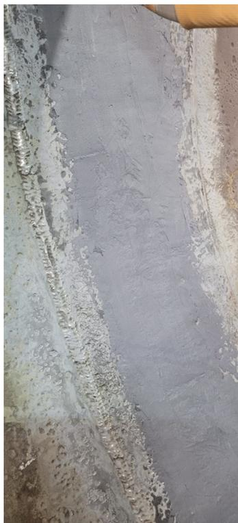
After surface preparation and rebuilding with Belzona 1311
