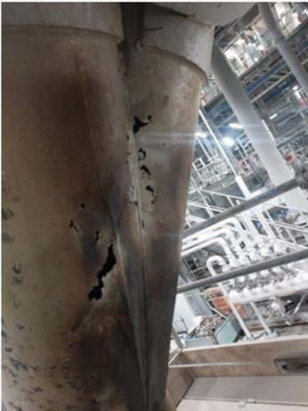
Ash chute had worn due to sliding abrasion
