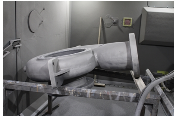
Surface preparation in grit blasting booth
