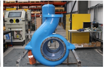
Belzona 1321 applied internally
