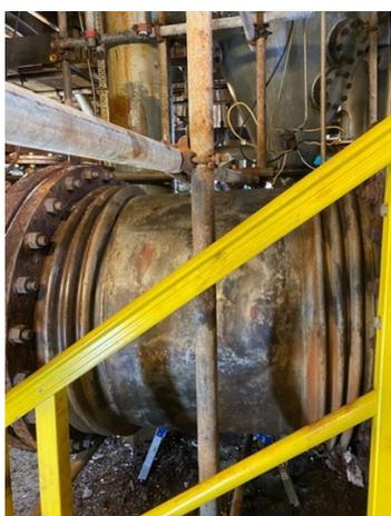
Worn and cracked bellows between two convolutions
