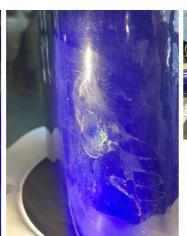
This was the most damaged area on the glass coated pipe. 1 coated pipe. 1/2" x 1 1/2" x 1/2"
