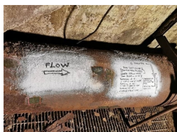
Corroded pipe with severe metal loss
