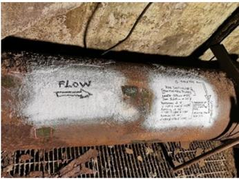
Corroded pipe with severe metal loss
