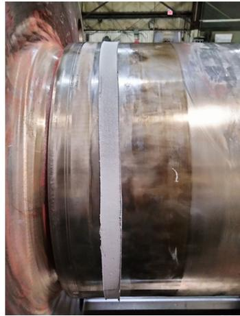
Belzona 1111 application finished and ready for machining
