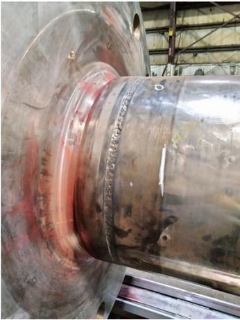
Shaft preparation completed for rebuilding
