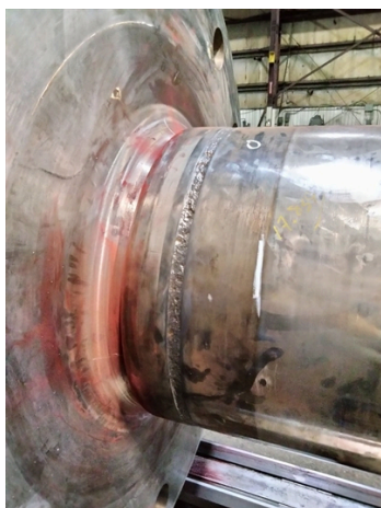
Shaft preparation completed for rebuilding
