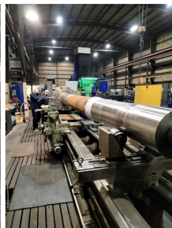
Shaft repair areas waiting on cure times so the machine shop can machine to the correct measurements.
