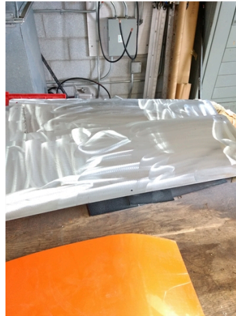
Surface preparation on the underside of the plate to be bonded
