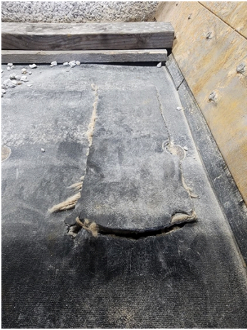
Original condition of the belt showing the large area of damage.
