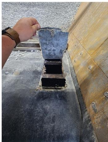
Lifting the torn flap of the conveyor belt to show the extent of the damage.
