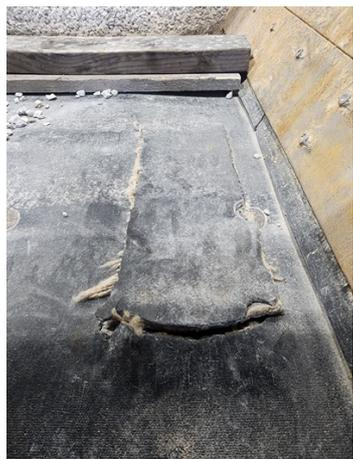
Original condition of the belt showing the large area of damage.
