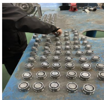
Metal former used to case nozzle inserts
