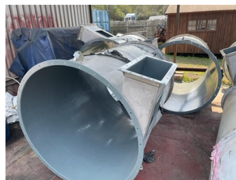
Cyclone internals coated ready for delivery
