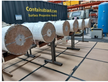
A total of over 3000 corks where required for plugging the faces
