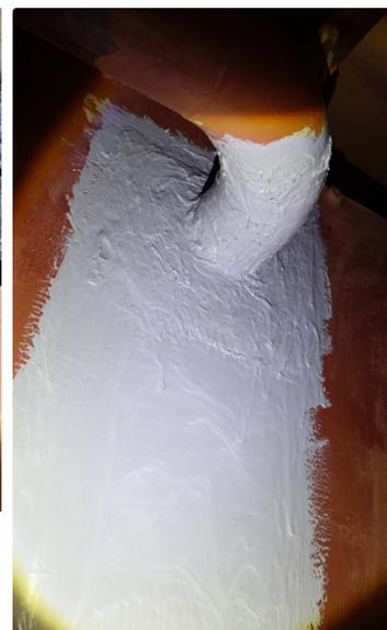
Surface coated with Belzona 1391T
