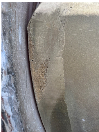
Damage to propeller
