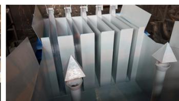
Application of the second layer of Belzona 1341.
