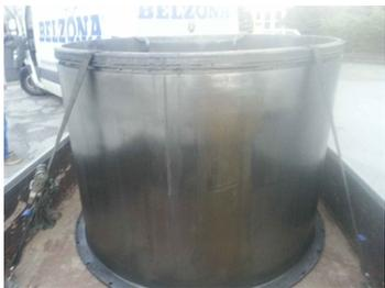
Damaged cylinder surface.
