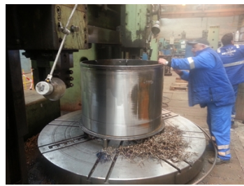
Centering of the piston in the machining device, turning the surface around the entire circumference to a depth of 1.6 mm.
