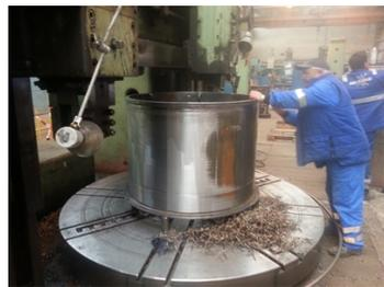
Centering of the piston in the machining device, turning the surface around the entire circumference to a depth of 1.6 mm.
