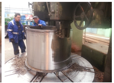
Final grinding and polishing of the surface to the nominal dimension and surface roughness
