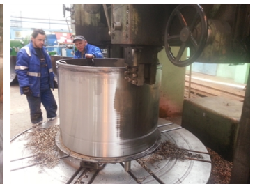
Final grinding and polishing of the surface to the nominal dimension and surface roughness
