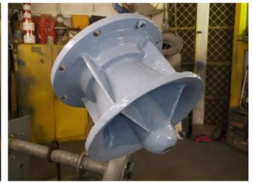
Protected with two coats of Belzona 1341N.
