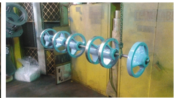
All six spiders completed with two coats of Belzona 1341N.
