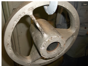
Grit blasted and ready for rebuilding.
