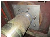
The gasket area former in place Application complete showing with Belzona 1111.
