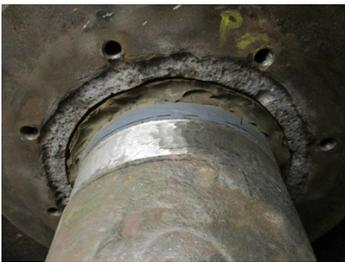
Showing the area of damage to the shaft and gasket surface prepped.
