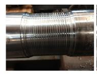
Shaft is mounted on a lathe. and the area has been machined down and roughened, ready for the application.
