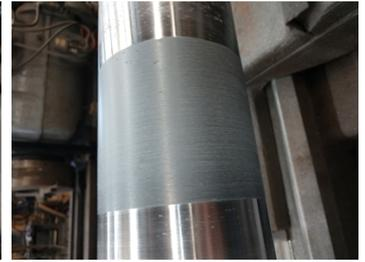
Application completed, fully machined, and dressed down with emery cloth.
