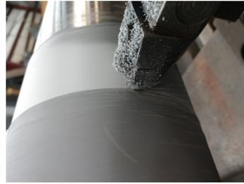
Machining the Belzona 1111 to the proper dimension.
