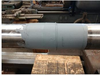
Belzona 1111 applied while the lathe was turning slowly.
