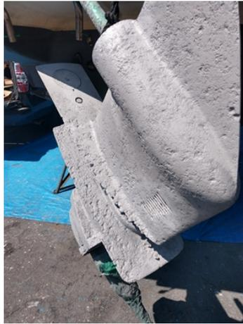
Up close, showing the erosion damage.
