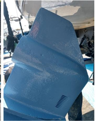
Belzona 1341 applied to protect the outdrives.
