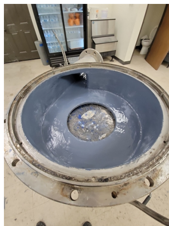
First coating of Belzona 1321.
