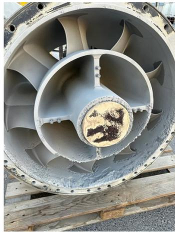
AFTER SURFACE PREPARATION BY GRIT BLASTING EXPOSING DEEP PITTING AND METAL LOSS.
