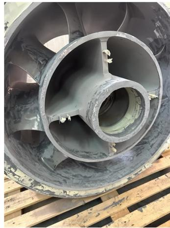
ALL DAMAGED AREA WAS REBUILT USING BELZONA 1311.
