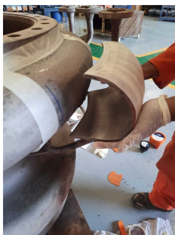
DRY FITTING OF THE PLATE PRIOR TO HOLE SEALING AND PLATE BONDING
