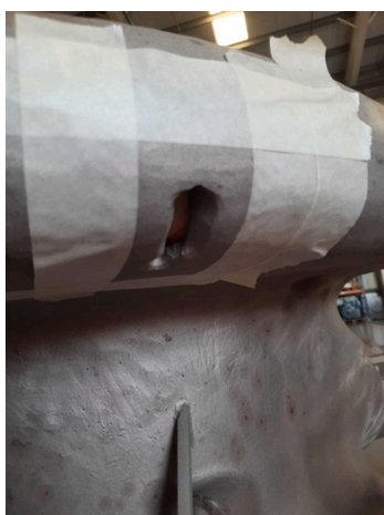
WIDENED CRACK LINE DRILLED ON BOTH ENDS.
