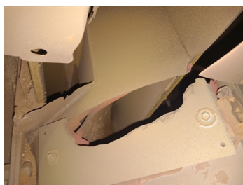
Internal view showing the totally worn away side plates where debris, dust and blast media can escape
