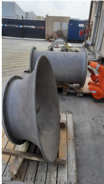
After surface preparation using grit blasting
