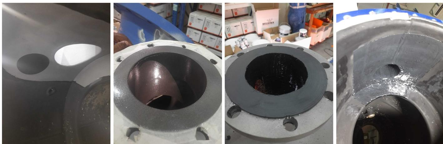
After surface preparation AND DURING SALT CONTAMINATION TEST
