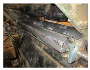
The roller with four sections taped off and hand ground, solvent washed and ready for application.
