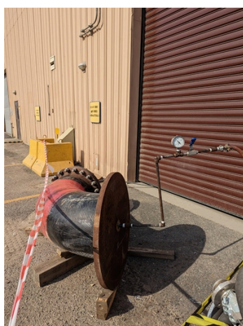
No trace of any leak or peel-off after the completed hydrotest.
