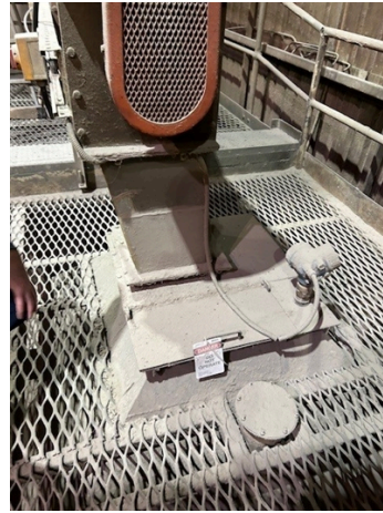
Access hatch from the top of the hopper allowing for one man entry.
