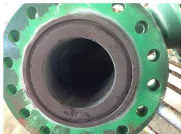
Damaged flange face due to high salt and H<sub>2</sub>S content
