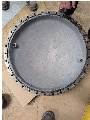
Metal resurfacing completed
