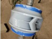
Impeller after the 1st coat with 2nd coat of Belzona 1341. Belzona 1341.
