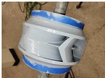
Impeller after the 1st coat with Belzona 1341.
