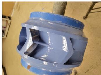
2nd coat of Belzona 1341.
