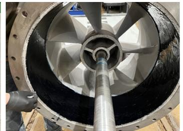
Interior of diffuser protected with two coats of Belzona 2141 ACR Elastomer (top coat of black shown)
