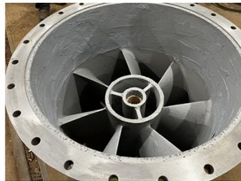
Metal loss rebuilt with Belzona 1111 Super Metal
