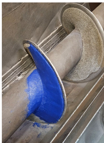
The damage after coating with Belzona 1818
