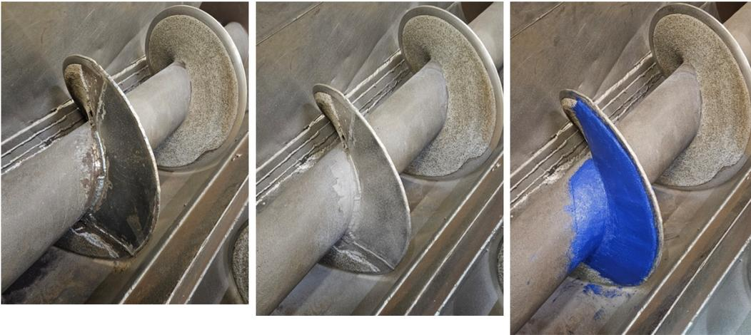
The damage before grit blasting    The damage after grit blasting    The damage after coating with Belzona 1818
