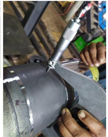
Smoothness, Tolerances checking (QA)
