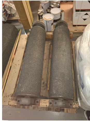
Belzona 1821 with incorporated grit applied
