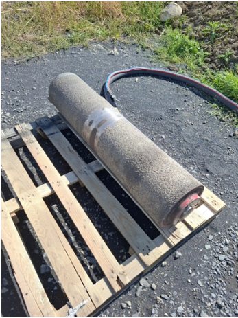
Failure of previous coating
