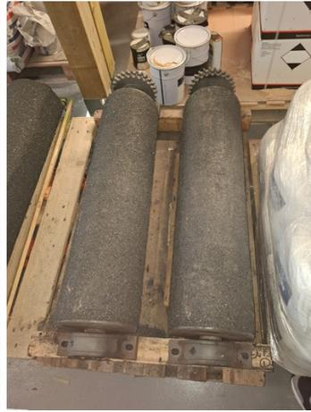
Belzona 1821 with incorporated grit applied
