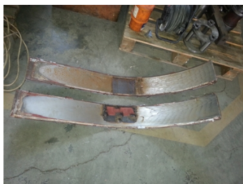
Surfaces prepared before applying Belzona products.
