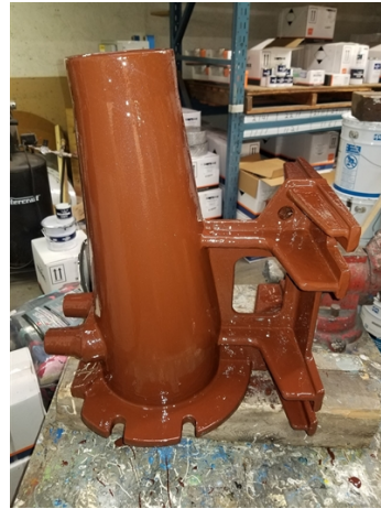
Belzona solution application.
