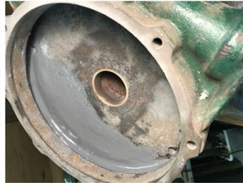
Inside of pump casing shows Belzona 1212 used to fill the crack and create a smooth finish for the water flow.
