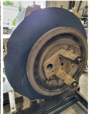
2 Coats of Belzona 1321 brushed to face to establish a long-lasting abrasion resistant finish suitable for the maintenance cycle.
