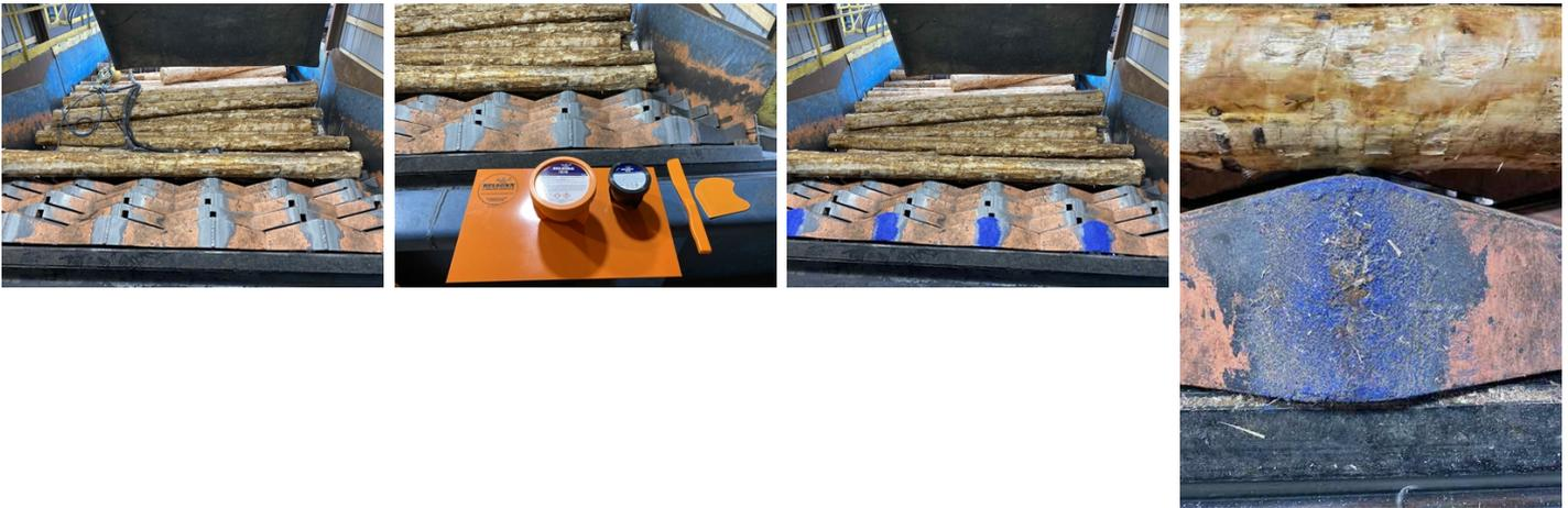
Steel grit blasted at welds that would frequently wear away.
